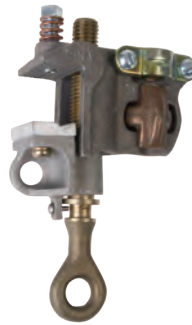
G336335J Aluminum body, Serrated jaws, Bronze eyescrew with fine threads, Bronze pressure-type terminal
