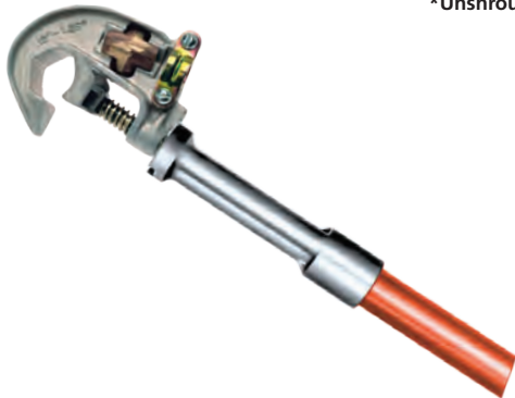
C6000386 *Mounted Clamp Aluminum body, Serrated jaws, Bronze eyescrew with Acme threads, Bronze pressure-type terminal
