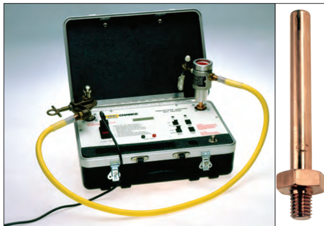
Optional Straight Stud Terminal T4033159 for testing grounded-parking-stand temporary grounding sets.
