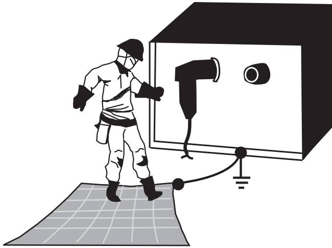
Use of a Conductive Mat to Develop an Equipotential Zone Figure 11-10
