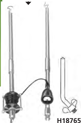
Extension Resistors, as installed
