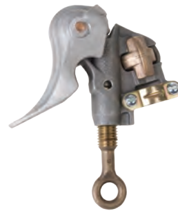
G36221 Aluminum body, Smooth jaws, Bronze eyescrew with fine threads, Bronze pressure-type terminal
